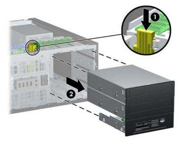
9. Gently slide the drive into the uppermost available bay until it snaps into place. When the drive is properly inserted, the drivelock will secure it. Repeat this step for each drive.
